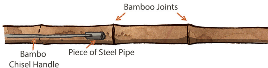
Figure 6-10: Joining Two Pieces of Bamboo
