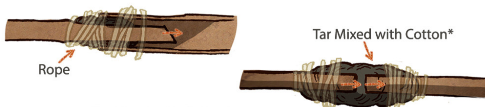
Figure 6-10: Joining Two Pieces of Bamboo
